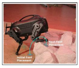
Fig. 1. An example where the swing foot trajectory is collision-free, however other parts of the swing leg (in this case the elbow) will be in collision with the terrain during the swing.
